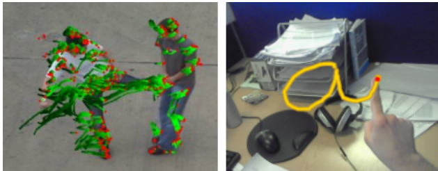
Figure 1. Two examples of spatio-temporal trajectories. On the left, trajectories representing human motion. On the right, a character 'a' written in the mid-air using the fingertip and an egocentric sensor.
